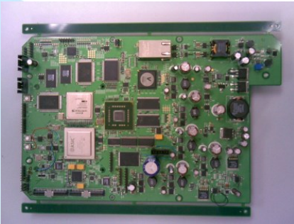
== Wimax Base Station Controller
