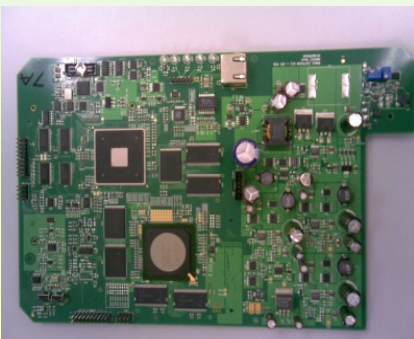
== Wimax + WiFi Base Station Controller
