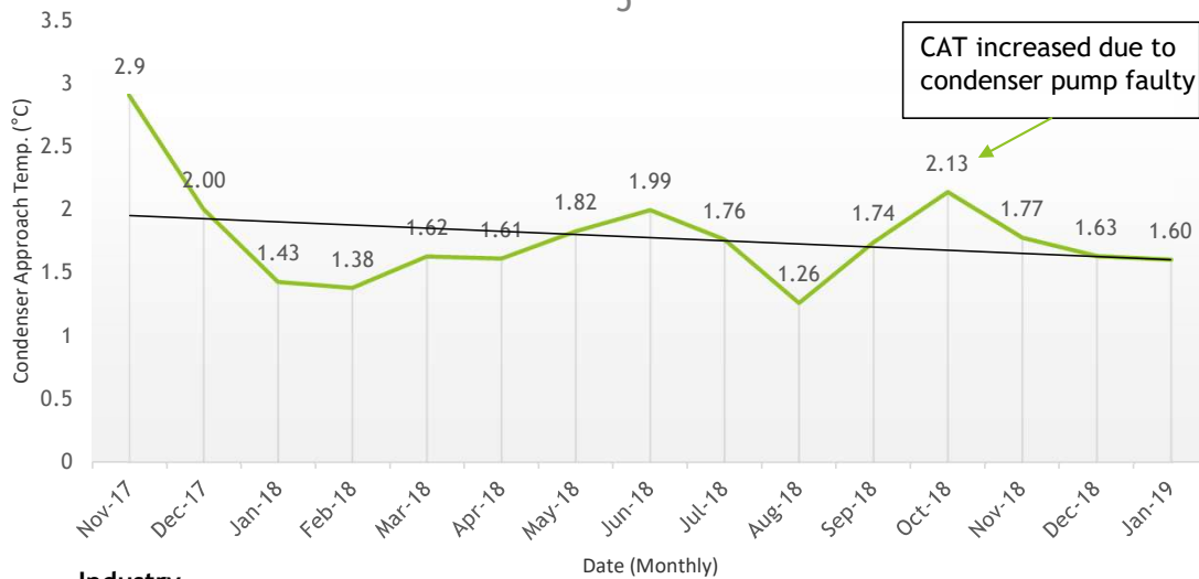
Condenser Approach Temp. @ Barry Callebaut Malaysia Chiller 5
