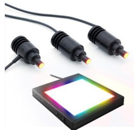
Ultra-high brightness SWIR coaxial spot light specially designed for Myutron SWIR Telecentric Lens series. Available wavelength in 1050nm, 1100nm, 1450nm and 1550nm. For complete system setup, you will need 3 items: SWIR coaxial spot light + MPP48W-C2 controller + resistor box. Input Voltage is DC15V max. 4A.
