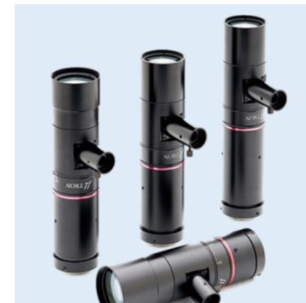
Suitable for SWIR image sensor up to 1", our SWIR telecentric lens is specially design to transmit SWIR 950nm~1800nm. It is possible to capture differences and defects that cannot be seen in visible ray.
