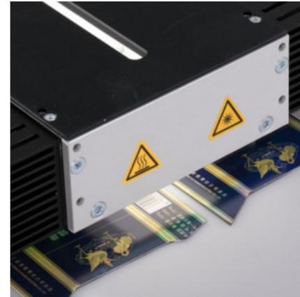
The Corona II family offers a wide range of lighting for line scanning in 4 settings: Dark Field, Bright Field, Tube Light, and Coaxial Module. All lights are available in different LED color: White (5500 K or 3500 K); Red (632 nm); Green (520 nm); Blue (452 nm); IR (850 nm or 940 nm); UV (395 nm). Module length available from 170mm to 1360mm in steps of 170mm.
