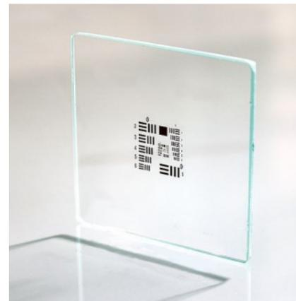
Machine vision applications are often expected to deliver high accuracy in alignment or measurement. A physical object showing the pattern arrays which are fixed spaces is called a calibration target, produced with a very high accuracy to ensure the generation of a transformation with a certain degree of accuracy.
